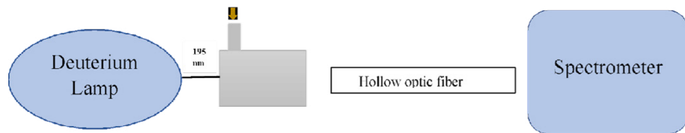
Simple schematic representation of three main components in the device. A deuterium lamp source produces light of 160-400 nm wavelength. A gas cell where a breath sample is introduced. A spectrometer to measure the absorption of light.
