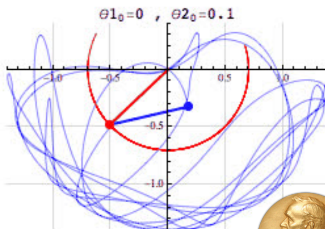
Chaos shown by the double pendulum with a slight difference in the starting angle of one of the pendulums. The paths are seen to be very different, especially at long times.
