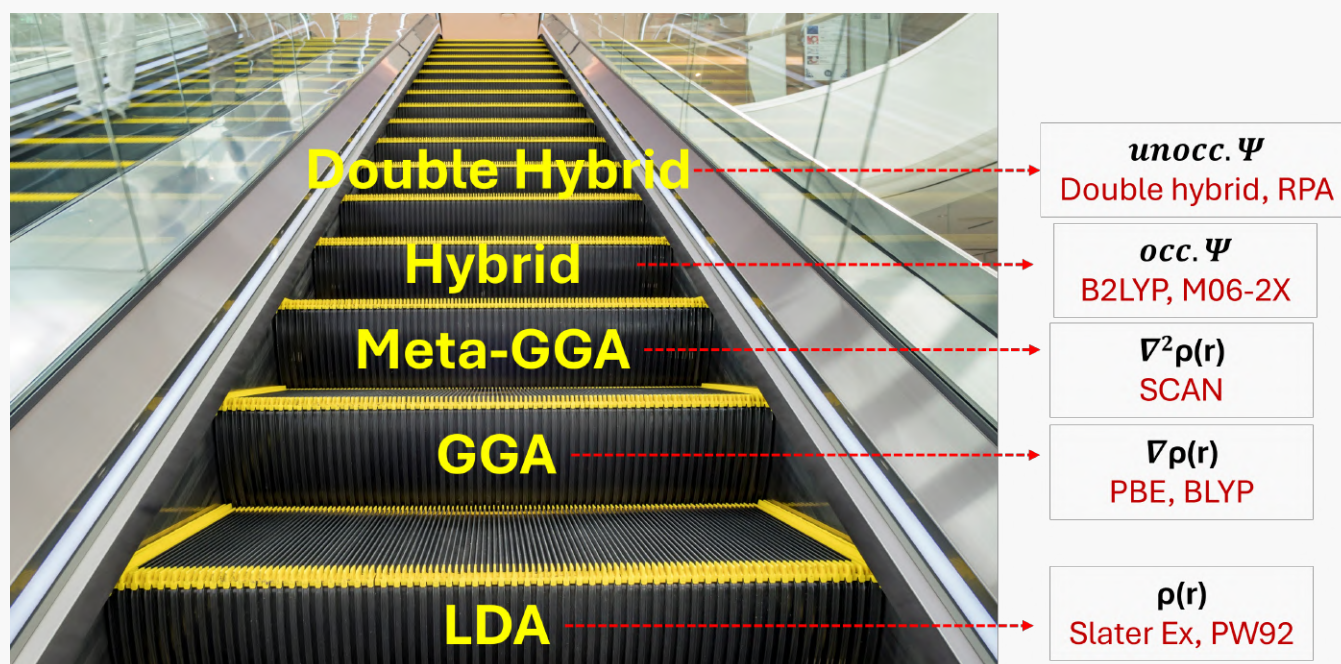
FIG 2 : Schematic representation of Jacob's ladder in DFT, approximations from LDA → GGA → meta-GGA → hybrid → double hybrid, showing increasing accuracy.
